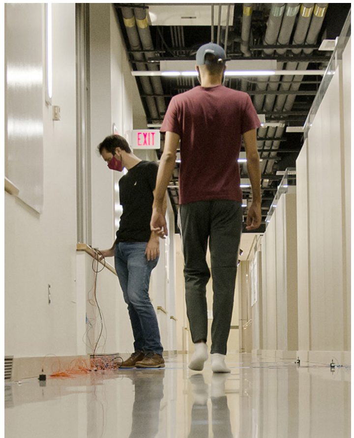
Rodrigo Sarlo and Rafael Gonçalves test gait monitoring via floor vibrations.
